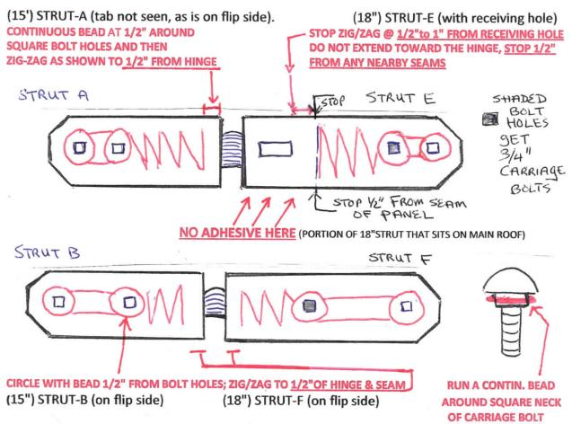
FLIP YOUR 'ASSEMBLY' RIGHT SIDE UP AND GENTLY POSITION THE SQUARE BOLT HOLES OVER THE DRILLED HOLES (drop a temporary carriage bolt in to help line up and hold in place if needed, or use masking tape). Apply gentle pressure to seat the Assembly and wipe away any XS adhesive.
